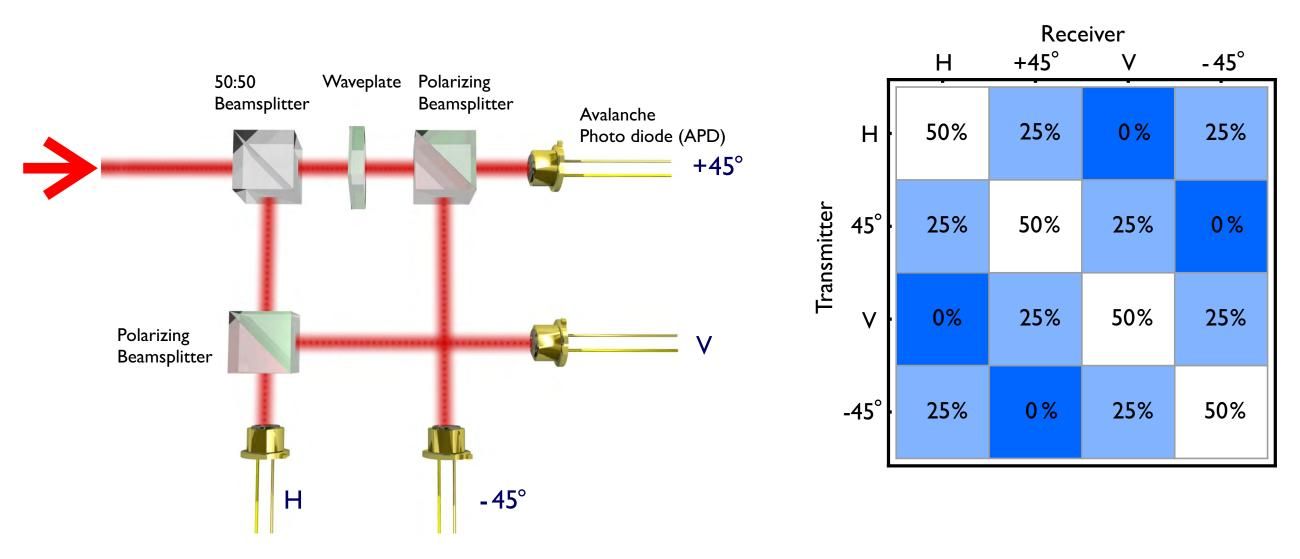
After all measurements the sender and the receiver can discuss on a public channel in which basis they have measured. First they discard all measurements which were not measured in the same basis and compare their number of detection events.
